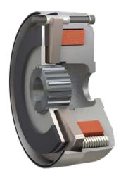
The ROBA-stop<sup>®</sup>-M safety brakes are designed for adverse ambient conditions. They are completely enclosed around the outer diameter and comply with Protection IP54 in standard design. Increased protection types are thus easily realisable. They cover a braking torque range from 2 to 1,600 Nm.
