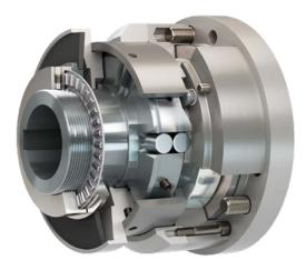
On the EAS<sup>®</sup>-reverse, the use of cup springs with a negative characteristic curve causes an instant drop in torque. This prevents the so-called pumping or breathing of the clutch. This generates low wear on the disengagement mechanism.
